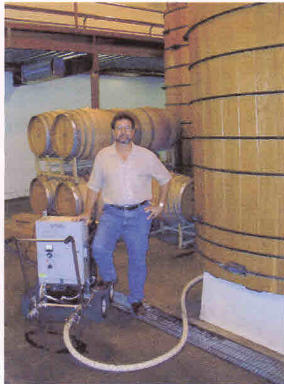
Dana DeLuvio at J Vineyards and Winery ready to move the ozone generator from the barrel room to the filler for CIP sanitation.
